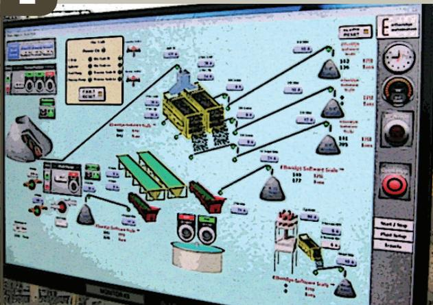
A plant that is totally automated runs with information from every component – including screens, bins, crushers, and conveyors. The automation software has more information than the operator and makes decisions on the fly about how much to alter speeds of specific components as needed to increase production. With interlocked components, the automated plant has the ability to shut down quickly, in proper sequence, providing greater safety.
