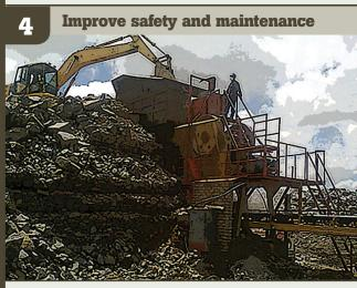
An automated plant will run at the optimal speed without overloading equipment. Because an automated plant is interlocked between all equipment, if there is an issue, it can shut itself down quickly in the proper sequence. Most stages can run unmanned, reducing the overall amount of manpower required and taking the plant from two or three operators down to a single operator. The system can also see maintenance issues and alert the operator before the plant breaks down.
