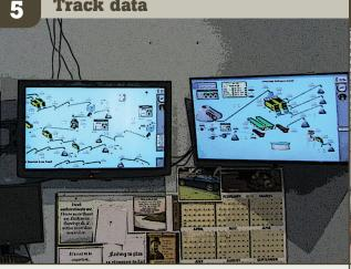
Automation allows operators to track productive and unproductive time. Managers on a regional or national basis can see the entire system remotely, allowing them to ask questions of the operator. By tracking data trends, operators and managers alike can adjust the plant for better performance. Historical data tracking ultimately improves the bottom line for better production and lower costs.
